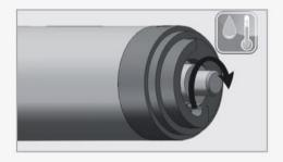
Assemble the regulation knob to the 38°C position.
